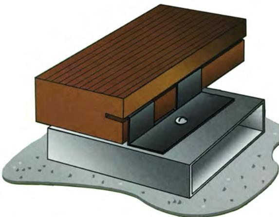
We then secure then plastic clip into the batten which in turn firmly holds the composite timber in place. This process is repeated to create a beautiful decking area with all screws and fasteners hidden away.
