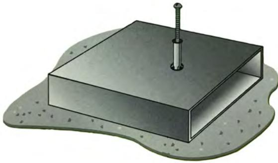
Our aluminium battens are held in place by 38mm Anchor bolts that secure onto the concrete surface below.
